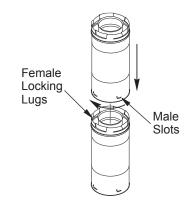
Figure 8 - Vent Pipe Connections
